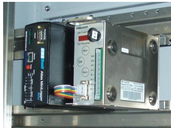
CDSRail MiniLogger with Bombardier EB/Track 200 digital TI21 receiver
